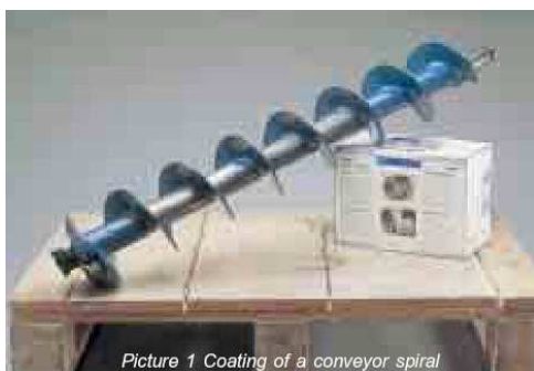
Picture 1 Coating of a conveyor spiral
